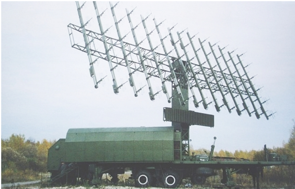
1Л119 Nebo SVU deployed (NNIIRT image).
