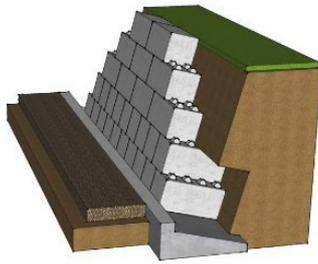
**Inclined Retaining Walls**
