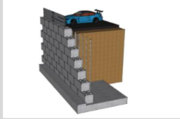
Reinforced Block Retaining Walls
