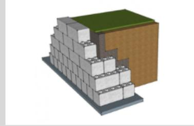
Gravity Retaining Walls
