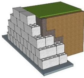
**Gravity Retaining Walls**
