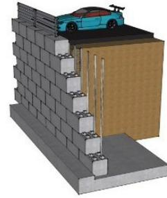
**Reinforced Block Retaining Walls**
