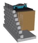
**Reinforced Block Retaining Walls**
