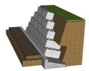
**Inclined Retaining Walls**
