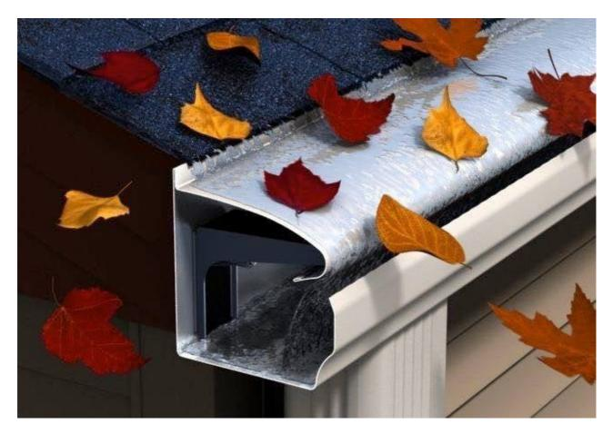
Their purpose is to divert the rain away from your roof and onto the ground in a controlled way.
