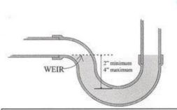
The weir of a p-trap <u>must</u> be below the top of the opening in the fitting that connects it to it's vent.
