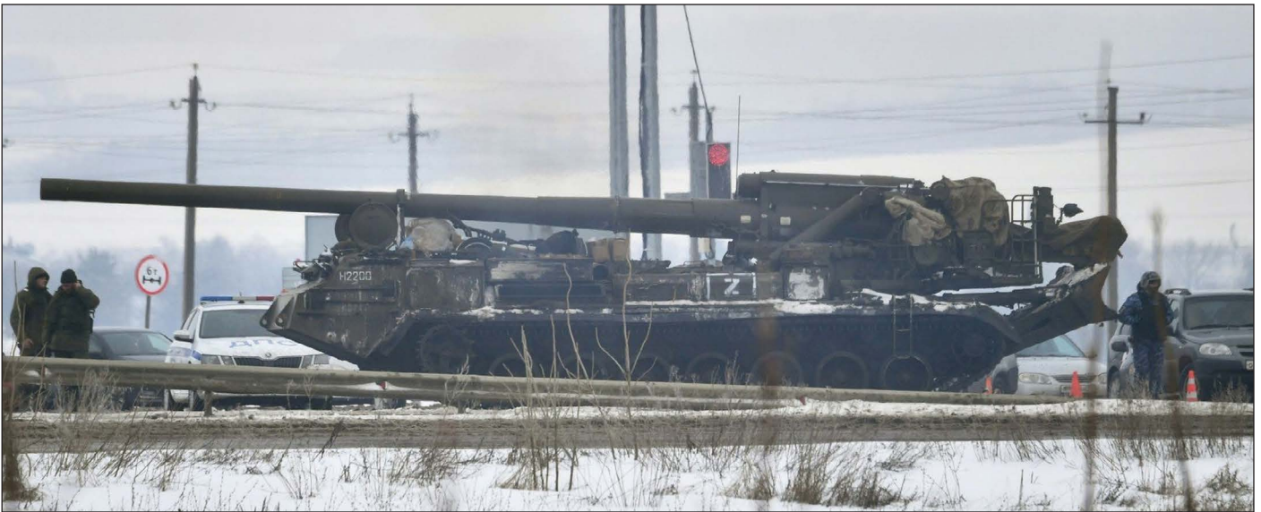
A 2S7 Pion – the heaviest self-propelled howitzer (203mm calibre) the VSRF deployed in Ukraine in 2022 – seen underway towards the Ukrainian border in the Belgorod area in early 2022. (Russian Internet)
