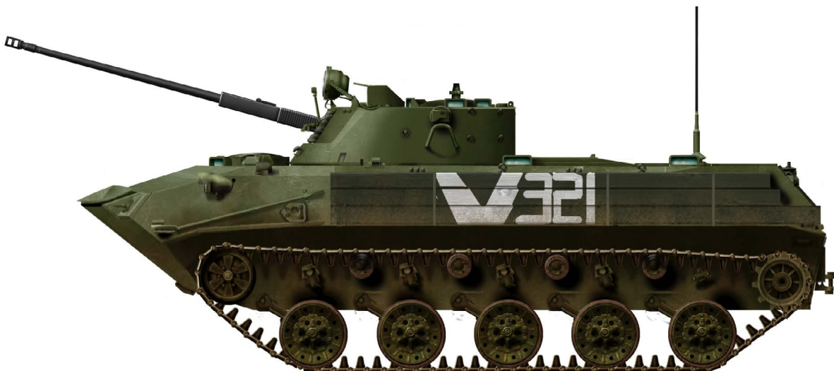
This BMD-2 of the 31st Airborne Assault Brigade is shown as it appeared in the Hostomel area on 24–26 February. The vehicle was left painted in its dark green overall colour, and had a number of metal or wooden planks added to the sides of the hull to bolster protection. The BMD-2's armour of welded aluminium alloy – 15mm thick at the front and lower hull, but only 7mm on the sides – proved highly vulnerable even to machine gun fire and attrition was heavy. (Artwork by David Bocquelet)
