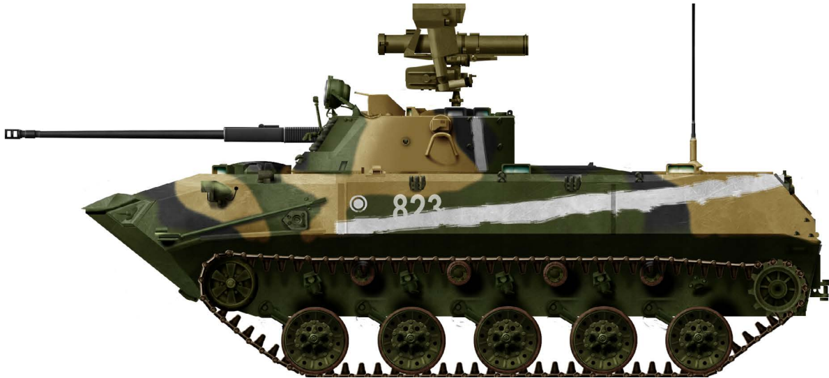
Still the most numerous armoured fighting vehicle of the VDV as of 2022, was the BMD-2. Dating back to the mid-1980s, it is armed with the 2A42 30mm autocannon, and a 7.62mm PKT coaxial machine gun. Many BMD-2s deployed in Ukraine in 2022 were also equipped with the pintle-mounted the 9P135M-1 ATGM launcher, shown above the turret. The BMD-2 has a crew of two and can carry six dismounts. This example was sighted in the Kherson area in early March 2022. (Artwork by David Bocquelet)
