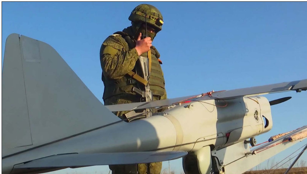
A serviceman of the VSRF preparing an Orlan-10 UAV for launch from a catapult. (Russian MOD)
