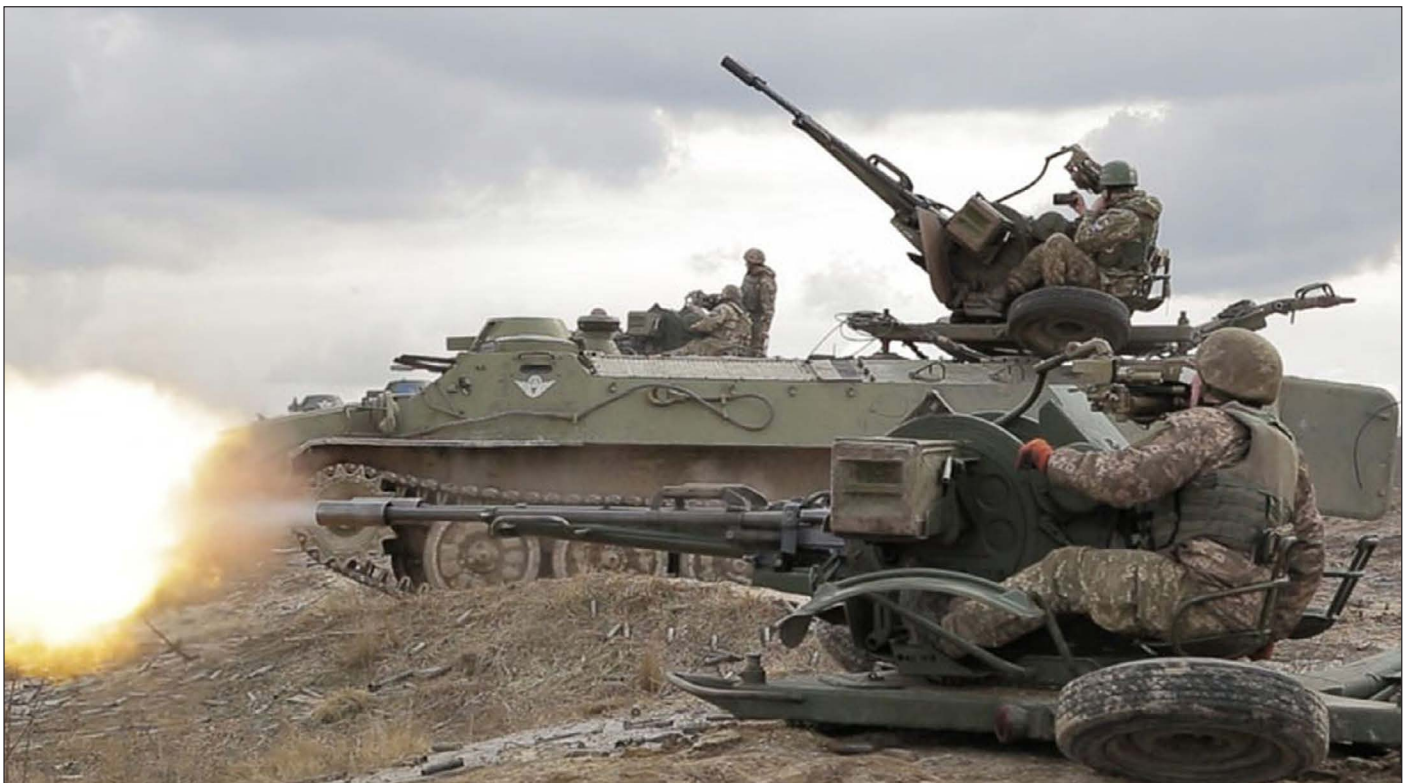
An MT-LB armoured personnel carrier, carrying a ZU-23-2 anti-aircraft gun on its rear deck, and a similar ZU-23-2 gun on the ground, both belonging to an airborne assault unit of the ZSU, seen during a pre-war exercise. (Ukrainian MOD)
