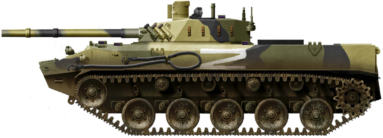
Airborne Assault units (VDV) of the Russian Armed Forces formed the spearhead of most operations in the first days of the invasion of February 2022. Like the rest of the VSRF, they were completely mechanised, and equipped with custom-designed light armoured vehicles. The most advanced of these was the BMD-4 IFV, weighing 13.6 tons, and armed with the 2A70 low-pressure 100mm rifled gun, the 2A72 coaxial 30mm cannon, and a 7.62mm PKT machine gun. The BMD-4 has a crew of three and can carry up to five passengers. This example served with a VDV unit assigned to the 35th CAA. (Artwork by David Bocquelet)
