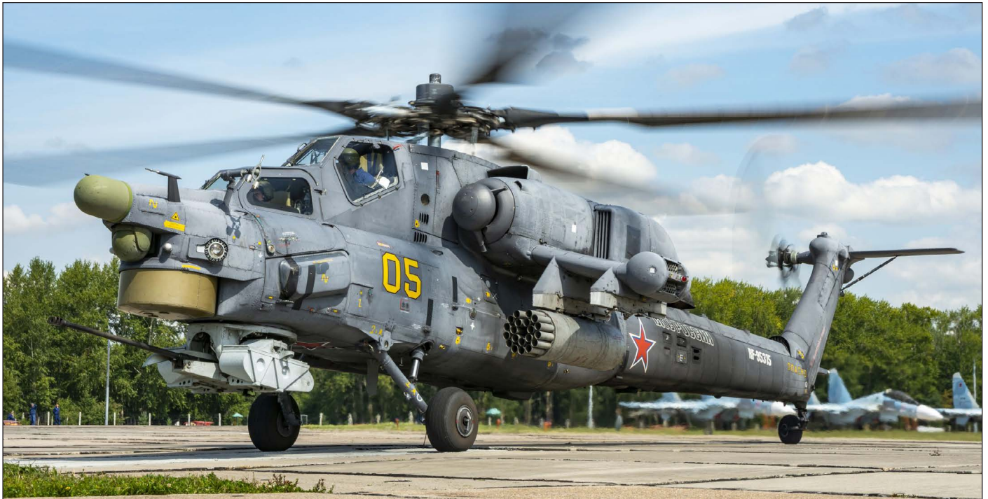
A front view of a Mi-28 helicopter of the VKS (serial RF-95315), seen at Kubinka AB in 2019, armed with a B-8M pod for unguided rockets. Notable is the turret with Shipunov 2A42 30mm automatic cannon. (Photo by Daniele Faccioli)
