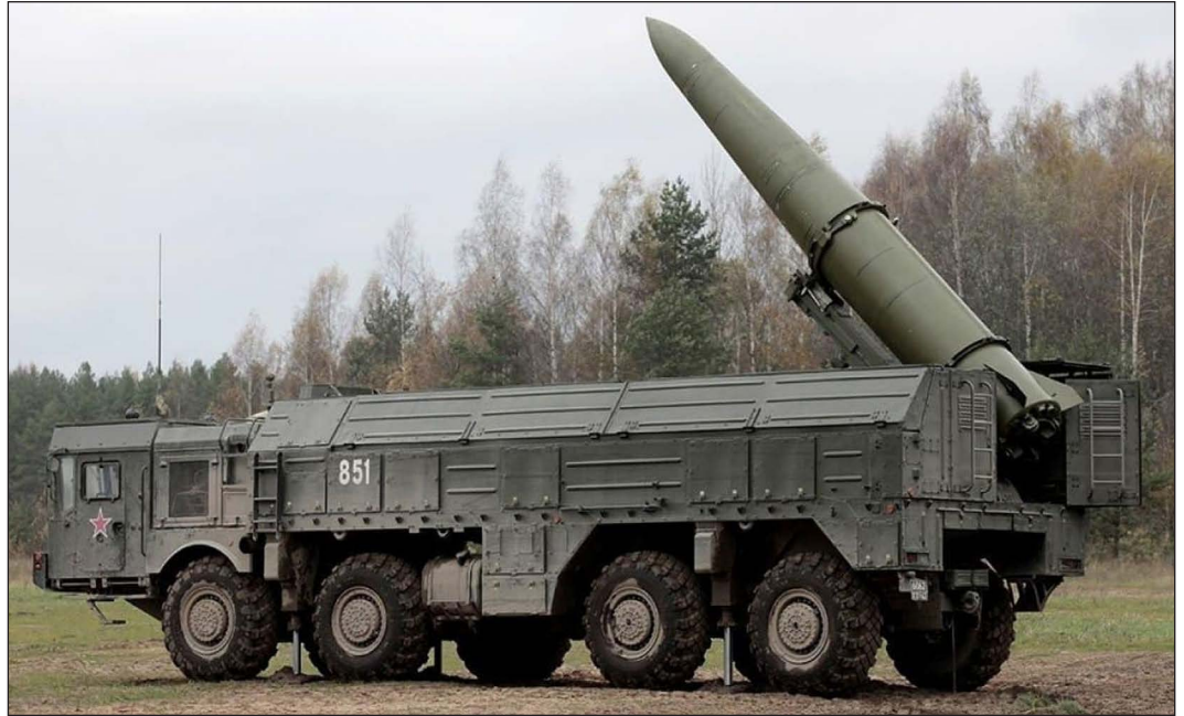
A transporter-erector-launcher (TEL) of the Iskander system of the VSRF, shown in the process of raising the missile into a firing position. (Ukrainian MOD)
