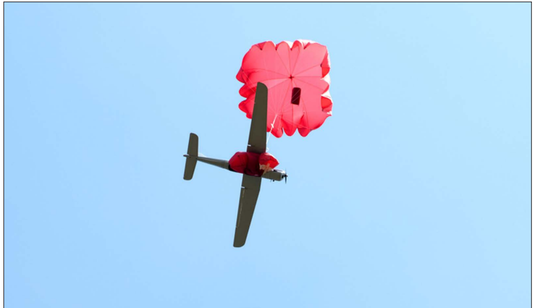
An Orlan-10 uses a parachute to aid its recovery following a reconnaissance flight. (Russian MOD)
